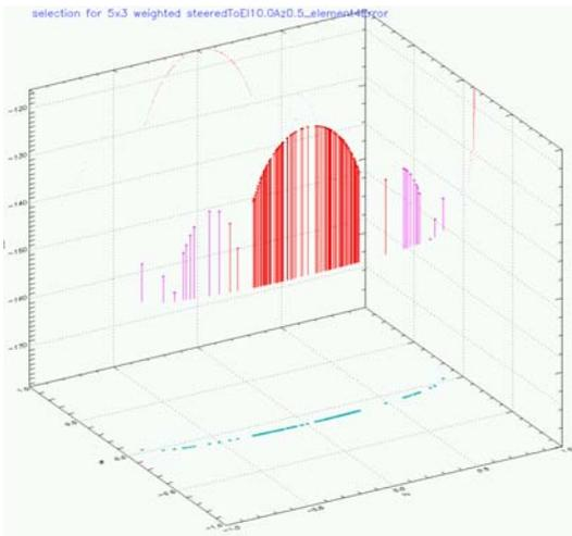
**Figure 6:** Measurement for the chosen set of basis vectors for the "5x3" array. The projection of the measurement points on the bottom plane show the associated base wavenumbers.
