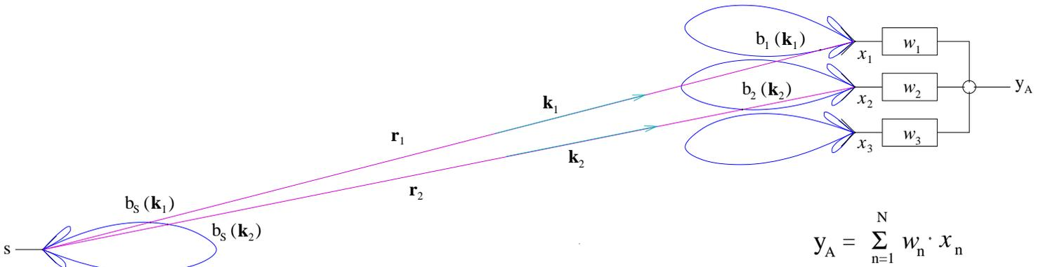
**Figure 1:** Diagram of the system used to describe the Weight Estimation Method with a sounding antenna S (bottom left) and the array to be characterized A (top right)
