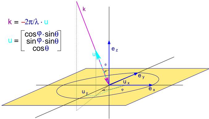
**Figure 2:** The coordinates of a wavenumber  $\mathbf{k}$
