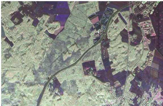
Figure 1 SAR image of forested region. Coloured composite of H- and V- channels, multi look image.
