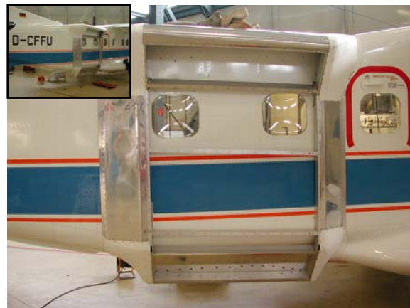
Figure 7 New F-SAR antenna mount attached to the right hand side of the aircraft behind the wing allowing 7 antennae to be integrated.
