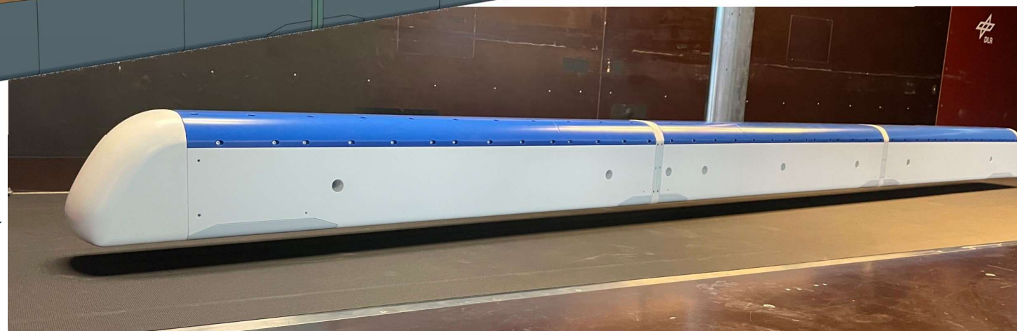
wind tunnel model, scale 1:20, on moving belt
