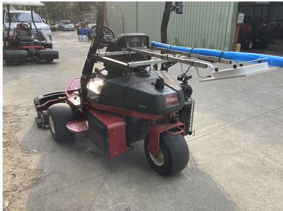
Figure 4. The L-band polarimeter mounted on the greensmower.
