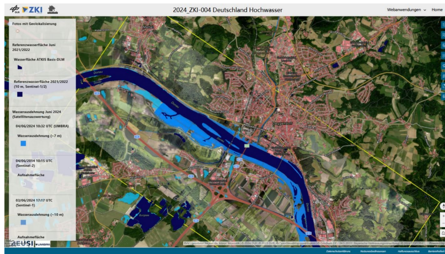
Fig. 4 Flood zones and affected areas in Passau, Germany. Flooded areas are shown in light blue, the reference water mask is shown in dark blue. Additional information (e.g. infrastructure and settlement areas) are shown in pink. Web-based viewer created by the authors using ArcGIS Experience Builder, version 3.24 [17]
