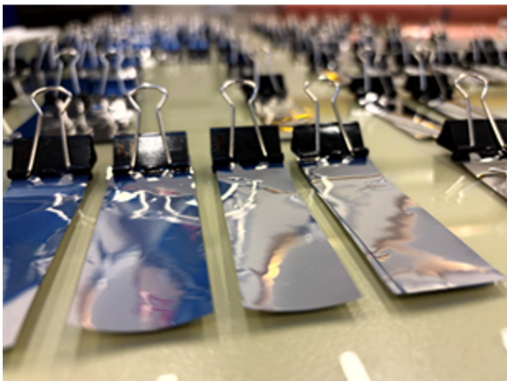
Fig. 7: Samples for preliminary testing (25 mm x 80 mm strips).
