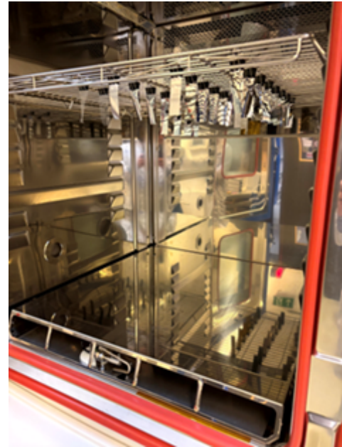
Fig. 8: Preliminary thermal cycling test in a climate chamber at DLR's Institute of Space Systems.
