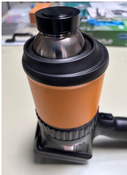
(b) Reflectance measurements with Surface Optics 410Solar / ET100. On top of the reflectometer is a light trap in order to absorb transmitted light e.g. for transparent drag sails.
