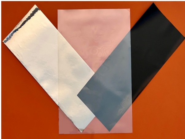
Fig. 1: Semi-finished products of ProFilm thin films. On the left an aluminized polymer film, in the middle a transparent film, and on the right a black non-transparent film.
