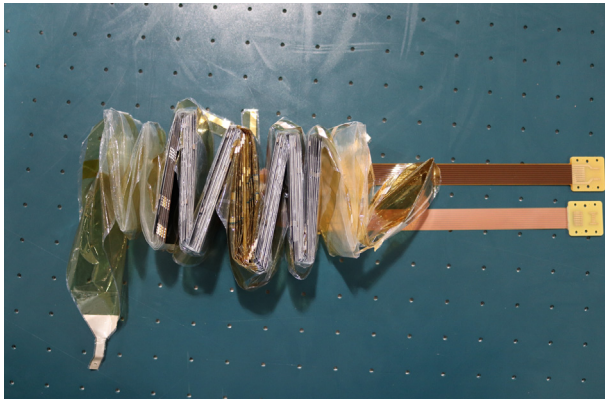
Fig. 15. The stowed blanket with the electrical interfaces on the right (FlexPCBs). One boom tip interface can be seen in the lower left corner.
