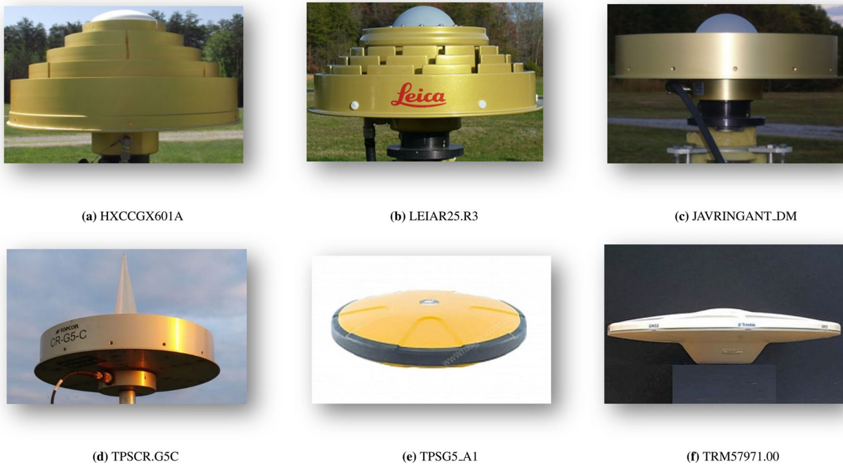
Fig. 2 GNSS antenna designs used in the campaign, such as 3D choke ring design (a–b), 2D choke ring (c–d), and integrated ground plane (e and f)
