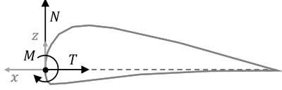
Figure 5: NTM loads applied at the leading edge in the CPACS coordinate system ( x downstream, y toward the right wing, z upward)
