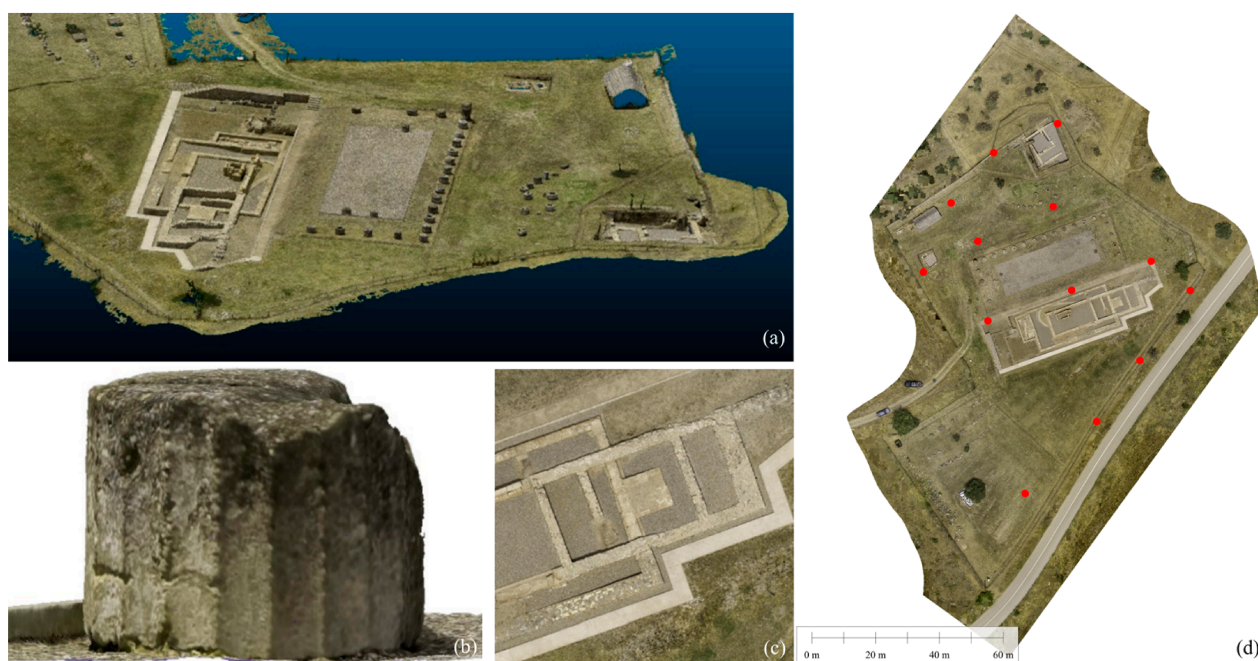
Figure 9. Geometric documentation of the Kalapodi sanctuary: (a) general view of the textured 3D model; (b) detailed view of the 3D model; (c) detailed view of the orthomosaic; (d) orthomosaic showing the spatial distribution of the 13 ground control points (GCPs, red circles) used for georeferencing.
