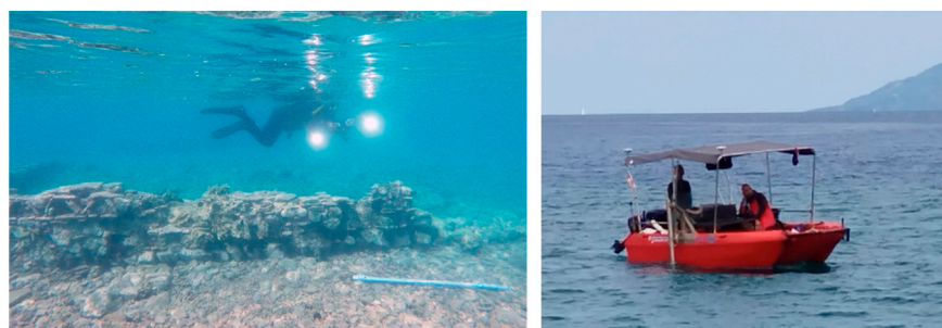
Figure 6. Fieldwork at the cultural heritage site of Ancient Epidaurus: underwater photogrammetric acquisition (left) and multibeam sonar survey (right).
