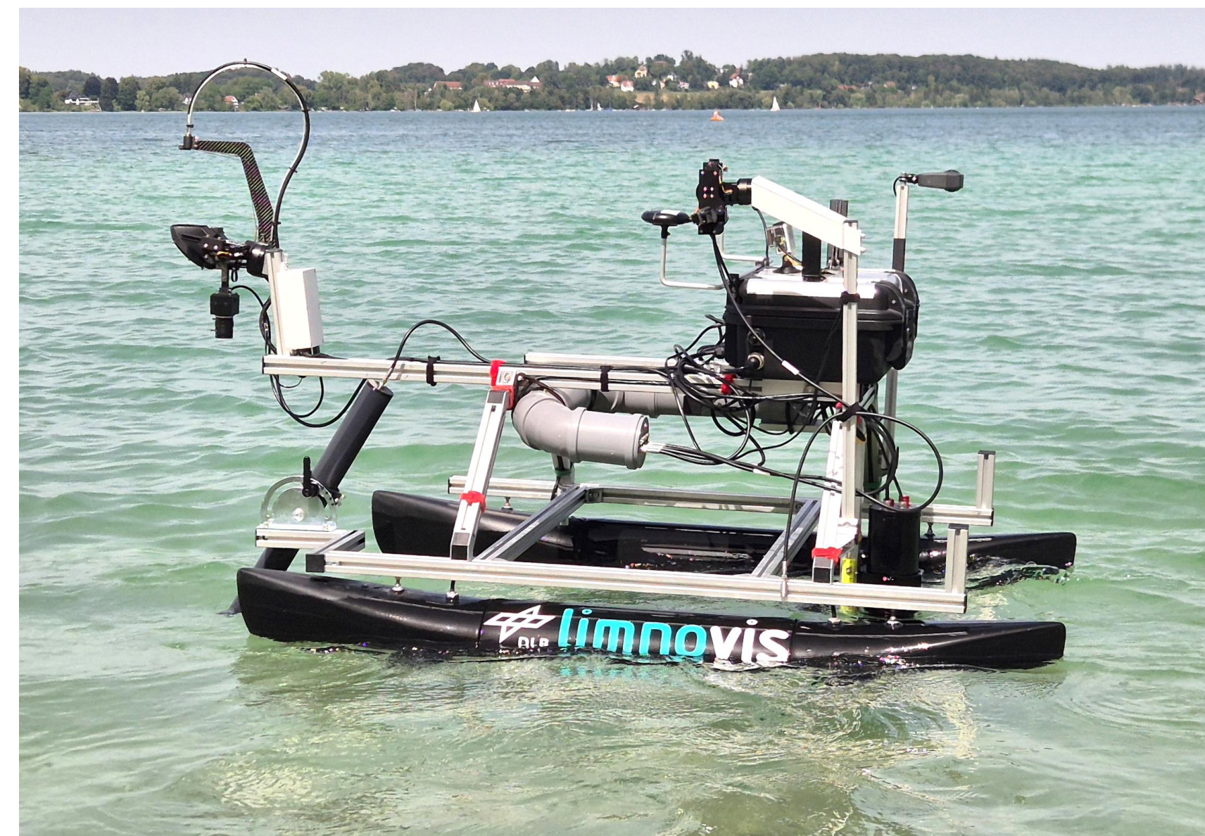
Fig. 2: The unmanned data acquisition platform LimnoVIS with its hyperspectral measurement system
