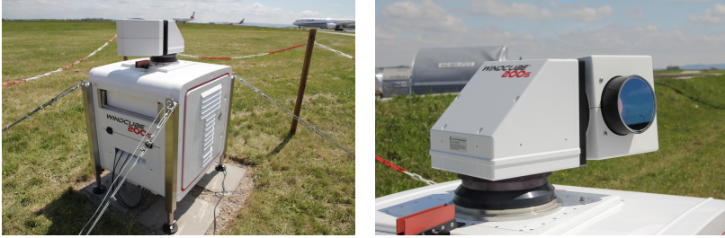
Figure 3.12: Vaisala WINDCUBE® 200s at Vienna Airport in 2019 on the airfield (left) with a close-up of the scanning head (right). Copyright by Frank Holzäpfel.
