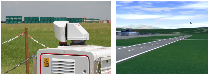
Figure 1.1: Photo of a Vaisala WINDCUBE® 200s lidar measuring at Vienna Airport in 2019 (left) and animation of a measuring on-ground lidar (right). The red line represents the lidar laser beam and LOS. Copyright by Frank Holzäpfel and DLR (2006), respectively.
