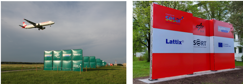
Figure 2.6: Experimental Plate Line below the glide path of landing aircraft at Vienna Airport in 2019 (left) and the permanent plate design exhibit at the German Aerospace Center (DLR) in Oberpfaffenhofen, Germany (right). Copyright by Frank Holzäpfel.
