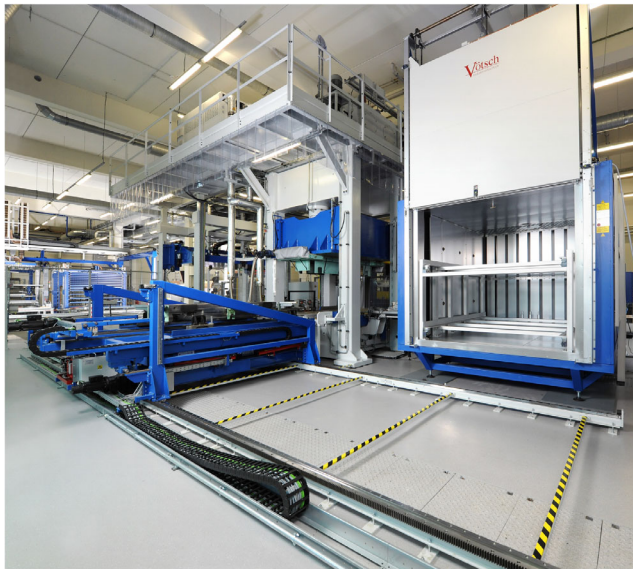
FIGURE 3 | RTM press as part of the automated “EVo” production line at DLR Stade, equipped with a mold-transfer-system connecting demolding station, press and oven. In this case, it will also be utilized for compression molding to process SMC material.
