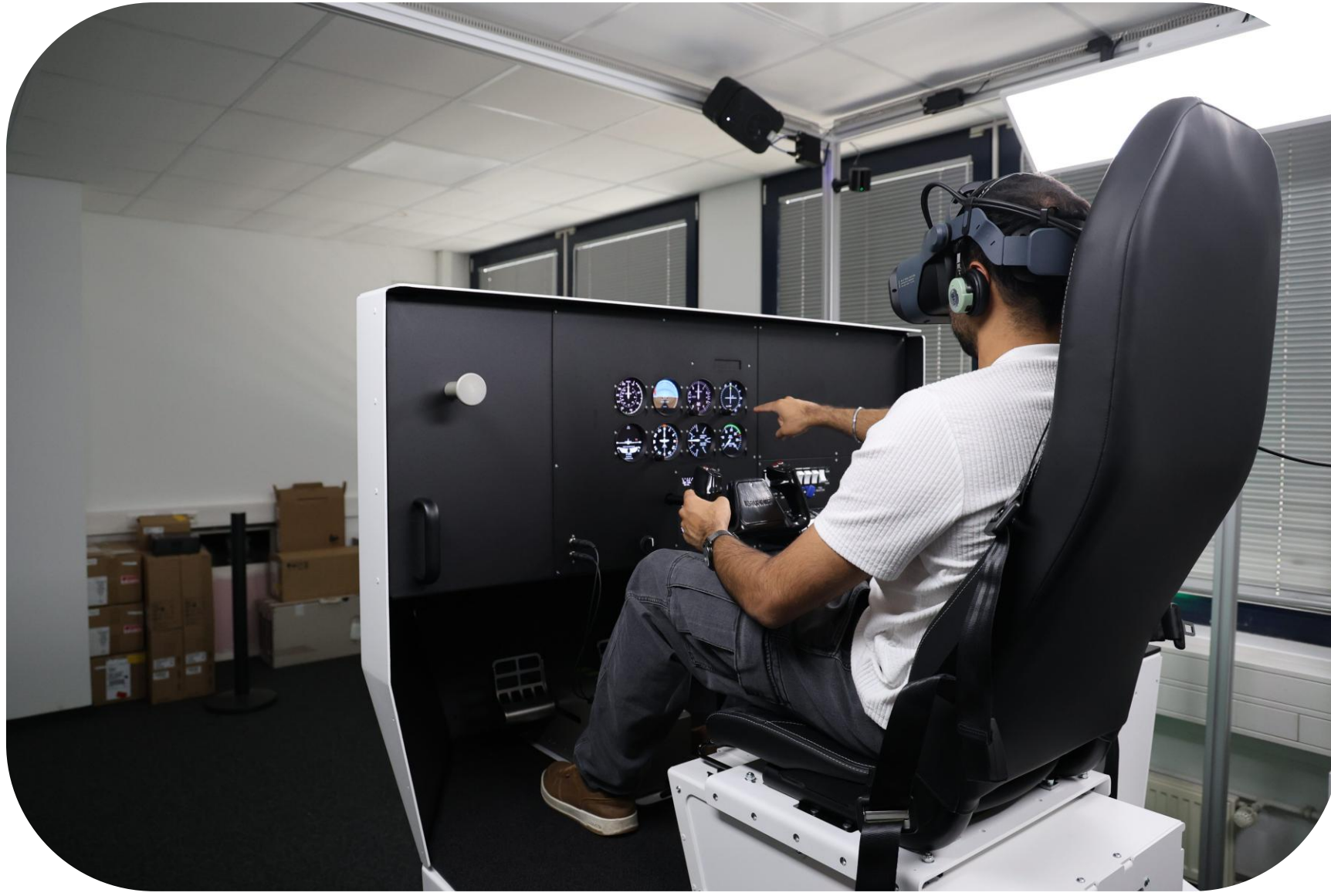
Figure 1. MR-Simulator of a PA-28 cockpit at DLR Würselen
