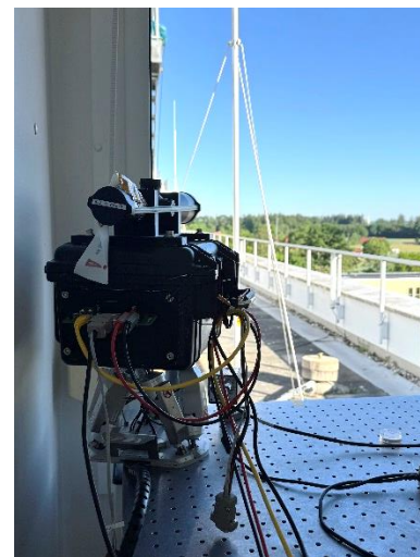
Figure 2: Terminal A mounted on the rooftop of DLR on the leftmost position in the container to avoid a treetop in the optical path
