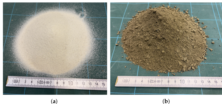
Figure 3. WF 34 (quartz sand) (a) and Syar (b). The particles of the Syar sand are heterogeneous and compressible, while the quartz sand is homogeneous. It does not deform easily under pressure.
