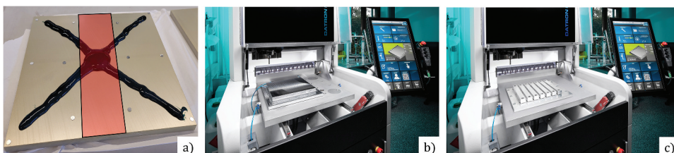
Figure 2. Steps in the TAST specimen manufacturing process: (a) Paste adhesive applied to plate A with spacers in place; (b) Outer contour milled; (c) Individual specimen bars with slots machined from the bonded plate.
