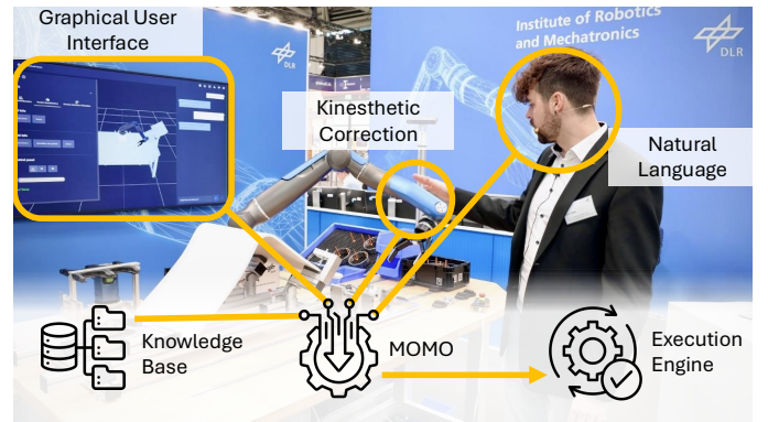
Fig. 1. Overview of the framework. The three interaction modalities (physical, verbal, and graphical) enable complementary skill adaptation, demonstrated on industrial robot tasks at a trade fair. The MOMO (Motion Modulation) module manages the different inputs and adapts the skill accordingly. The Execution Engine deploys the resulting trajectories on the robot.
