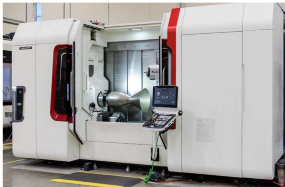
Figure 14. Virgin Orbit LT4300 Hybrid Manufacturing Machine [154].
