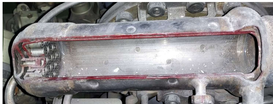
Figure 12. Section through the Isayev S2.720 gas generator.
