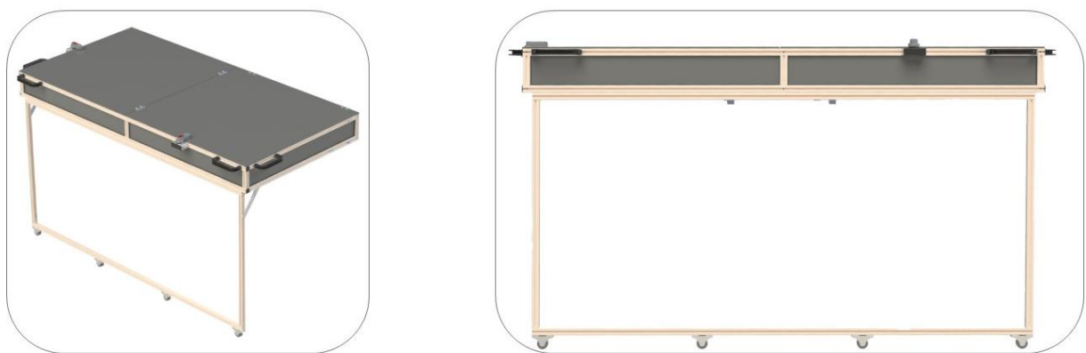
Figure 61: Substructure for the LAM-GTD platform prototype
