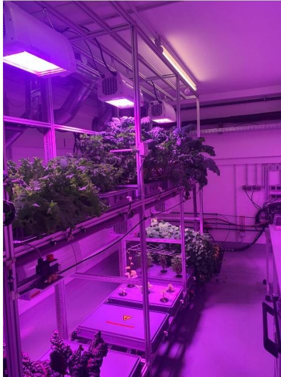
Figure 67: EDEN LAB two level plant rack
