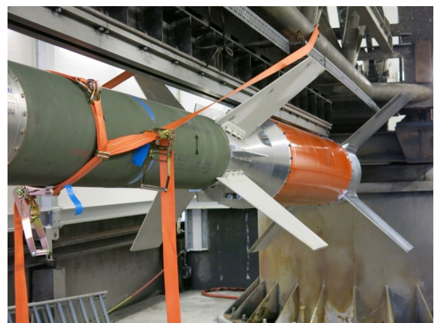
Fig. 33 Strakes between the fins of the second stage for improved aerodynamic stability
