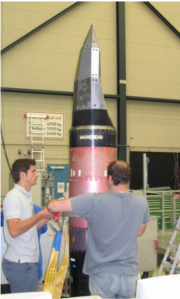
Fig. 24 The asymmetric forebody and payload of SHEFEX-1
