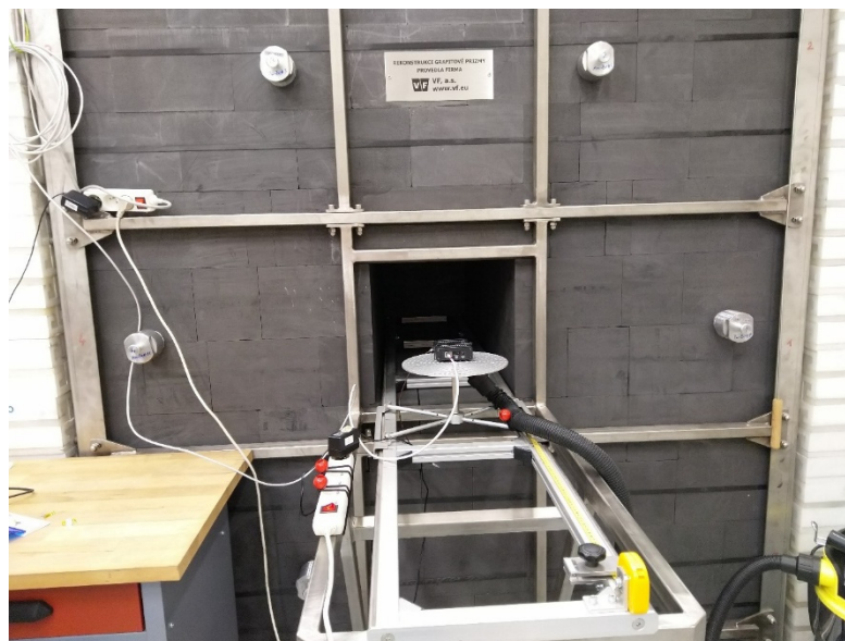
Figure 12. A graphite pile at CMI with 6 AmBe sources inserted around the detector in the middle.
