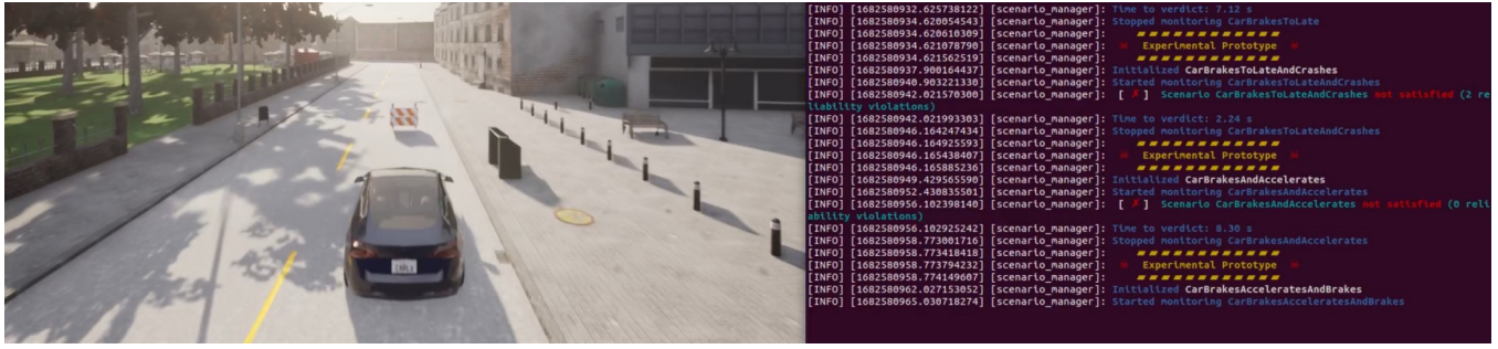
Figure 1: A simulation of an automated vehicle (left) performing a driving scenario that gets monitored (right).
