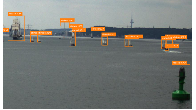
Fig. 1: Sliced detection results for an image snippet taken from a high resolution 19.6 MPix image showing detected object of varying scales.
