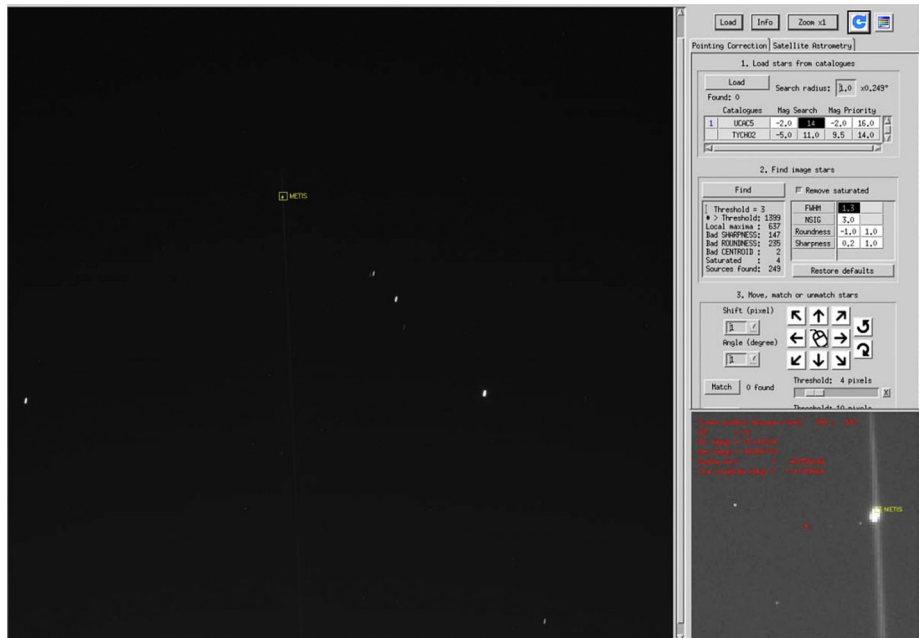
Fig. 17 Astrometric measurement of Metis from Cassini -ISS image N1356864415 using the Caviar software (Cooper et al. 2018). One can see the presence of stars in the background field that are used for calibration. Similar but more accurate measurements will be performed with the JANUS camera for the four inner Jovian moons
