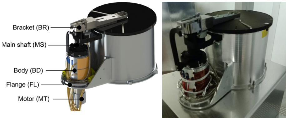
Fig. 14 COM subsystem together with its components: the stepper motor for controlling the position of the cover; the interface flange for fixing the mechanism to the baffle of the telescope; the main body where the mechanical parts for allowing the movements are present; the main shaft governing the vertical movement; the bracket holding the cover shield; the cover plate. Left image: rendering; right image: flight model
