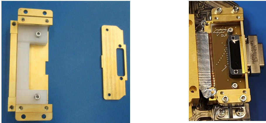
Fig. 24 Left: connector bracket and POM bushing. Right: assembled connector bracket
