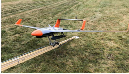
Figure 2. The Falk UAV on its launch rail; DLR (CC BY-NC-ND 3.0).
