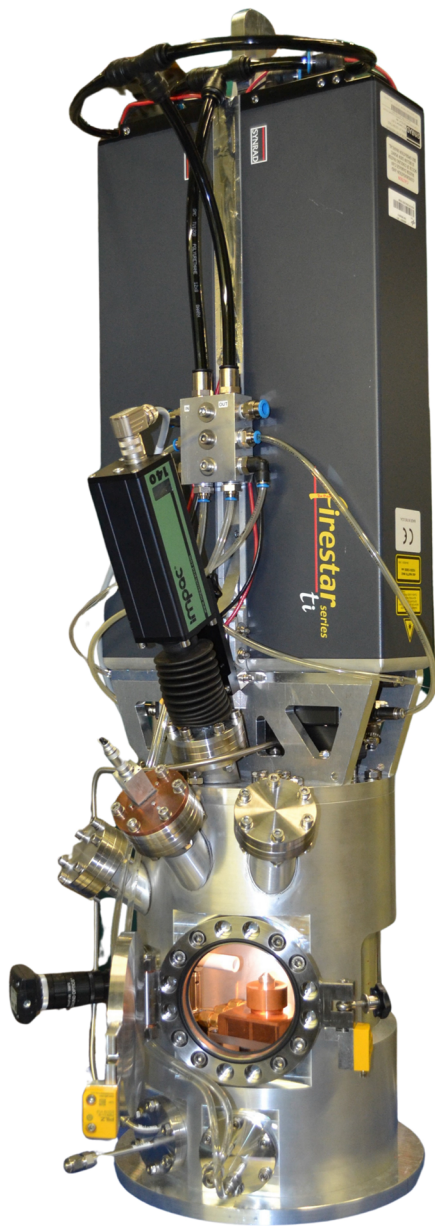
FIG. 1. Overview of the aerodynamic levitation apparatus. The upper assembly features two CO 2 lasers for sample heating, while the lower section displays the open levitation chamber with a direct view on the levitation nozzle. The visible attachments include a pyrometer (center, green/black) and a camera (left, black). The total height of the system is 1.12 m.
