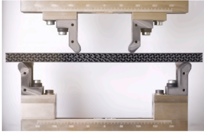
Fig. 7. Third-Point Loading test set-up with a sandwich specimen before testing.
