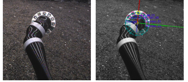
(b) Left: Jaco2 configuration with the AprilTag marker ring visible. Right: Same configuration with overlaid detection and offset w. r. t. nominal FK shown (dotted).
