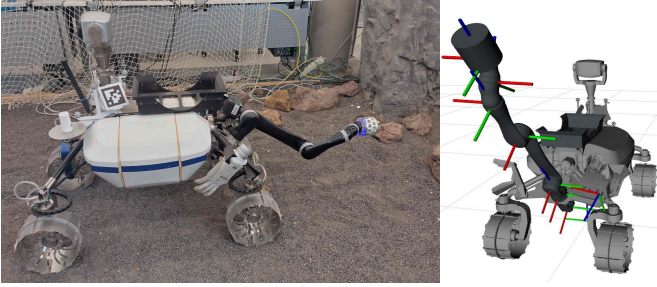
(a) Left: The rover in an example configuration while collecting the dataset. Right: Coordinate frames used during calibration and the rough field-of-view of the camera (blue).
