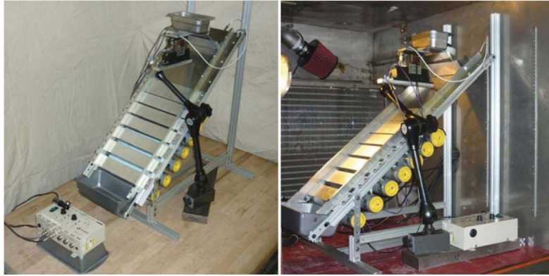
Fig. 2. Slotted Ramp Separator (SRS). Left: final assembly for testing; Right: Vacuum chamber in preparation for testing (Berggren et al., 2011).
