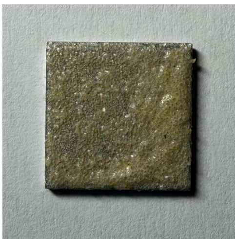
Figure A15: Representative photograph of sample 20251119-1 (KLPE 1:4 Ceramabind ® 880), showing the uneven and inhomogeneous coating surface.
