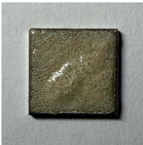
Figure A16: Representative photograph of sample 20260129-3 (KLPE 1:27 Ceramabind ® 880), showing the uneven and inhomogeneous coating surface.
