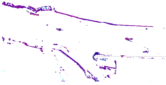
Fig. 2: Snapshot of one radar data station projected to latitude and longitude coordinates. Colored pixels are radar points encoded by their intensities (amplitudes). Blue triangles are AIS information.
