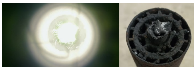
Figure 7. Experiment DLR-003: (left) Powder \beta ignites immediately after glowing. (right) A crust quickly formed, causing the burner to become clogged.
