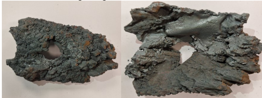
Figure 10. Images of the crust formation around the burner outlet: The top is shown on the left and the bottom on the right.
