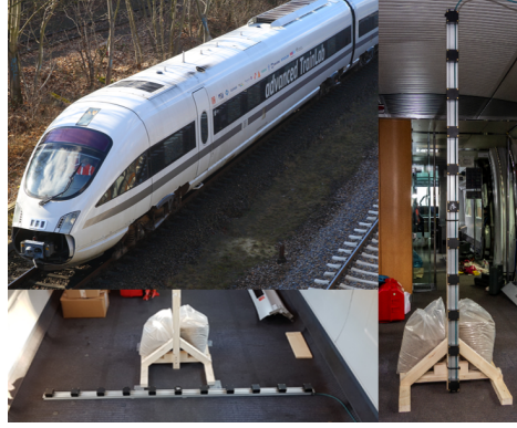
Figure 3.5: Advanced TrainLab of the Deutsche Bahn and magnetometer array with eleven elements in vertical (right image) and lateral (lower left image) mounting position.
