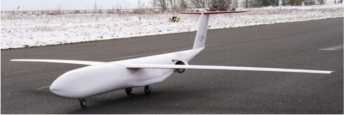
Figure 2: TU-Flex (FW configuration) flying demonstrator rollout. Credits: FMRA, 2025
