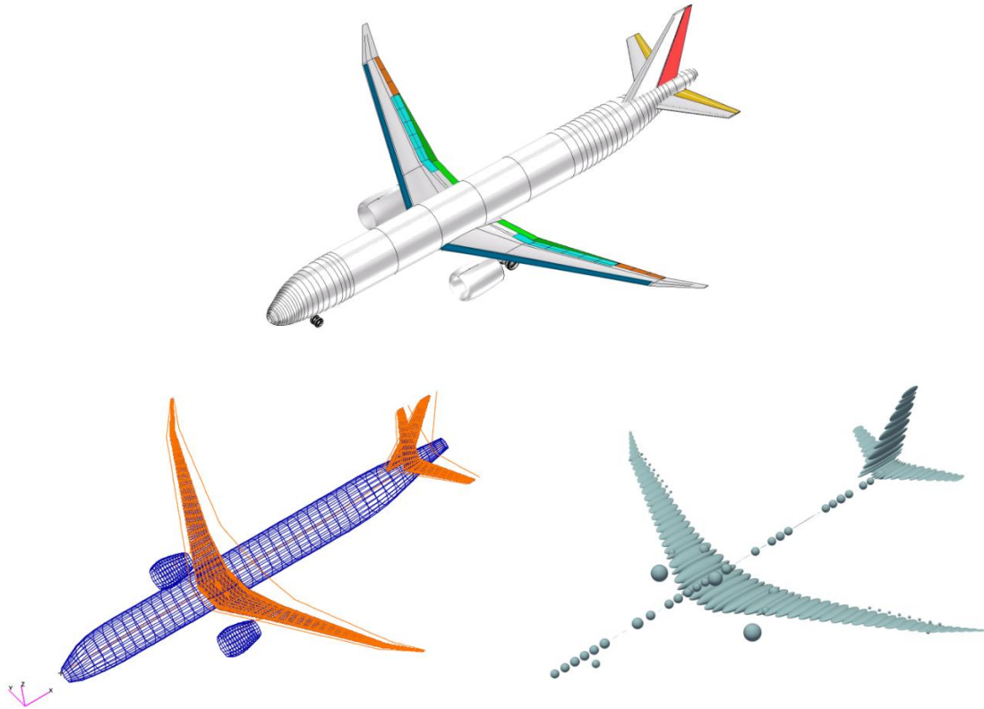
Figure 13. CPACS model (top), GFEM stiffness model (bottom left), GFEM mass model (bottom right) of D2AE
