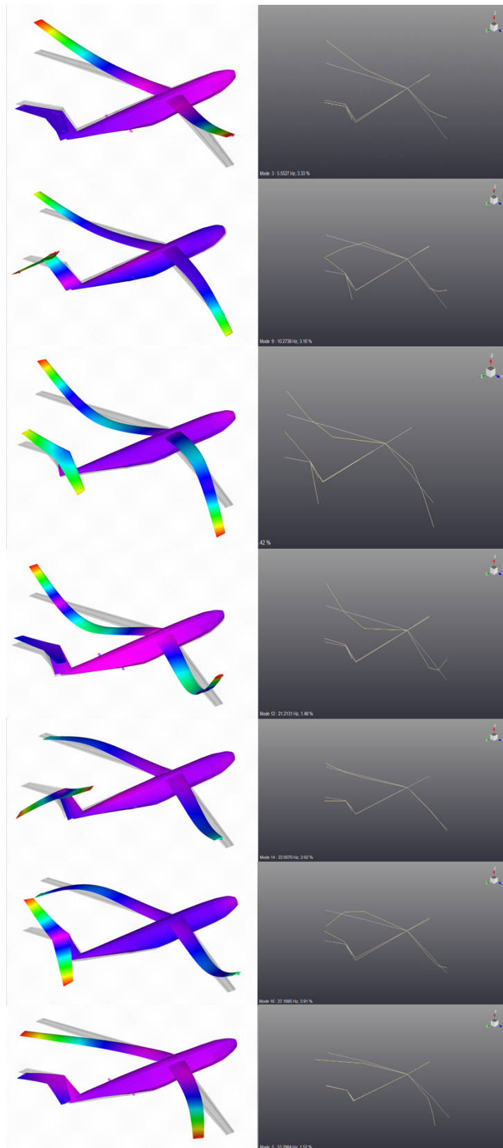
Figure 11: Comparison between the identified aircraft mode shapes and the FEM.
