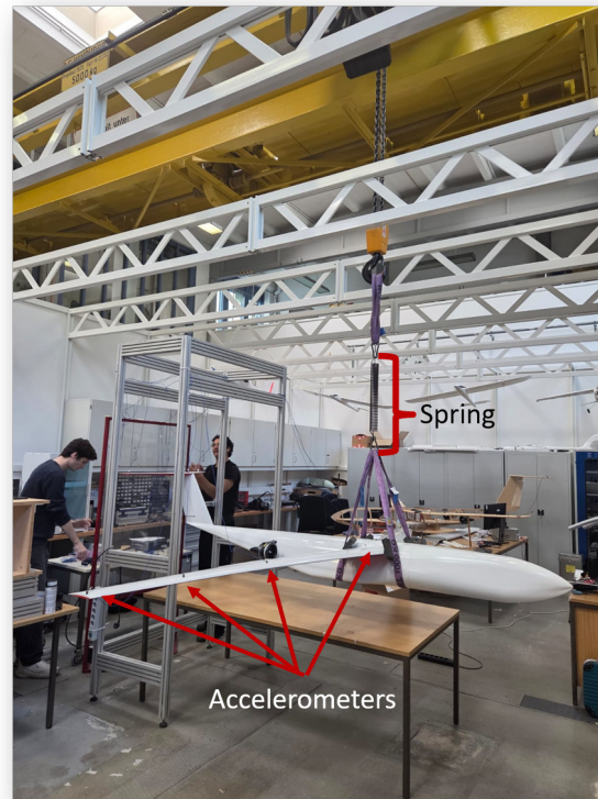
Figure 7: GVT of the full aircraft configuration.
