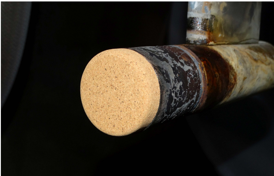
(b) Sample installed on the wind tunnel holder
