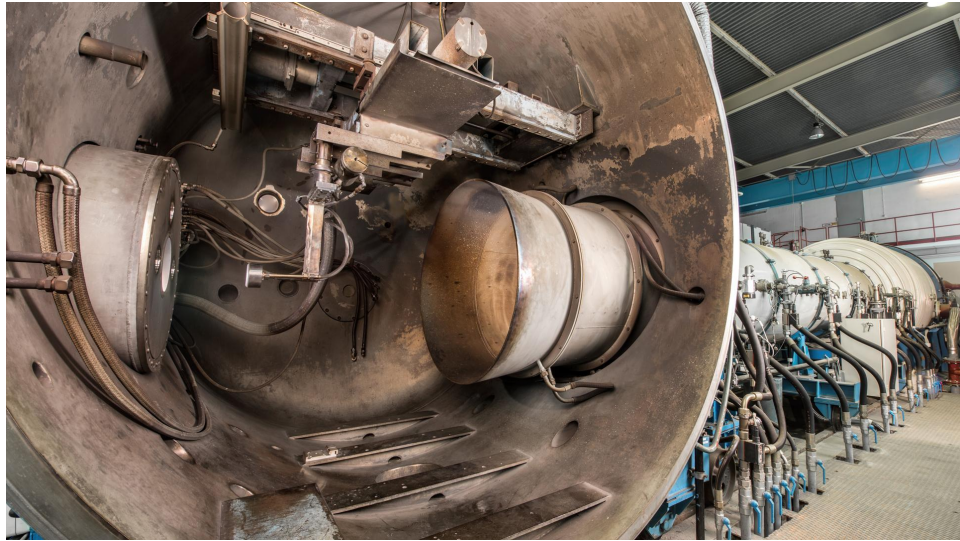
Figure 1.1: The L2K arc-heated wind tunnel with open test section
