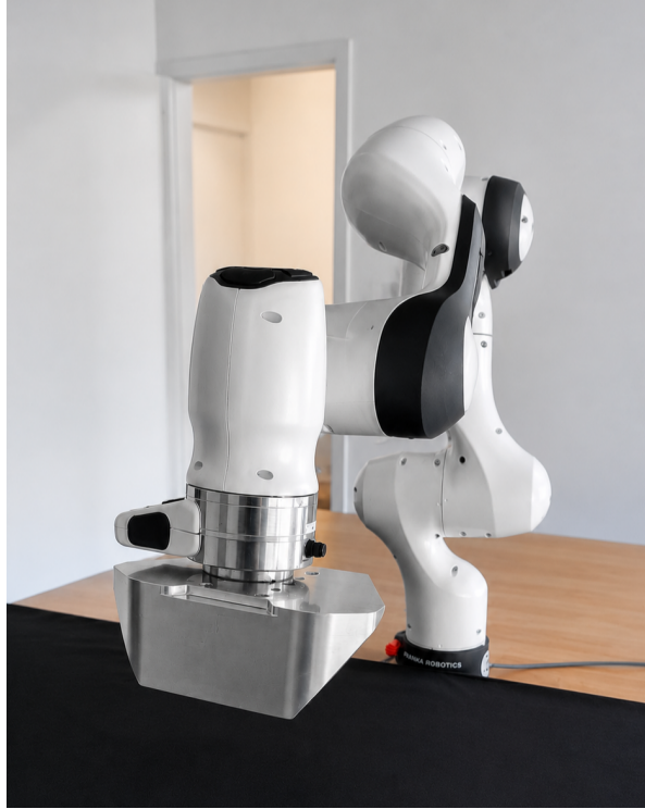
Figure 5.6.: Experimental setup for payload adaptation on the FR3 robot, with an unknown payload attached to the end effector.
