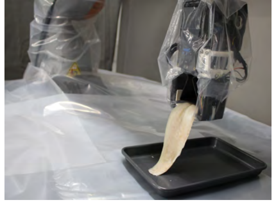
Fig. 12: Experiments with real fish, using food safe disposable protective cover for the gripper and the robot.
