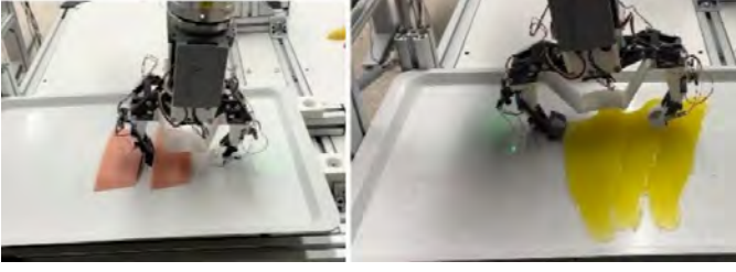
Fig. 7: Use of actuated scoopers for grasping in medium (left) and high (right) clutter scenarios.
