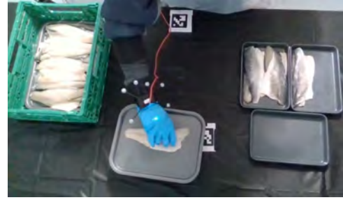
Fig. 2: Data collection in the fish experiments: Rokoko Smart-Glove, OptiTrack motion tracking, and Aruco markers.
