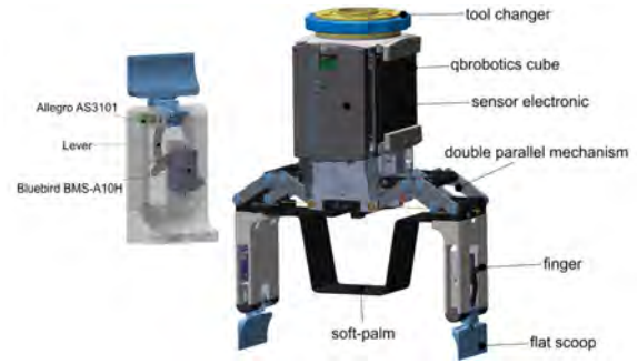
Fig. 5: Linear Scoop Gripper developed by DLR - left scooper actuation by servo over lever - ratio 1:1.2
