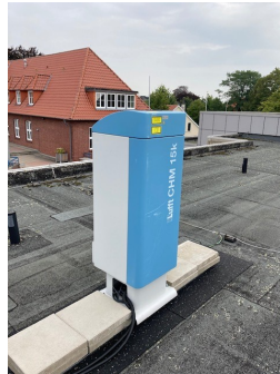
Figure 3.2.: Ceilometer Lufft CHM 15K [image taken from DLR Eye2Sky network]
