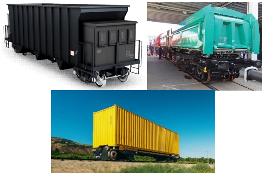
Figure 15.1 From left to right: IntraMotev "ReVolt", RZV Čakovec "Self-Prop Rail", Parallel Systems transport unit prototypes [1],[2],[3]
