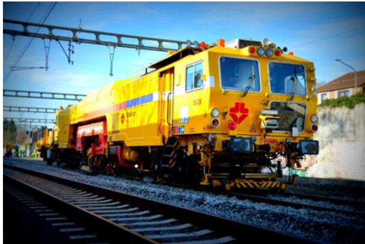
Figure 6.3 Leonardo inspection vehicle (Strukton Rail NV)
