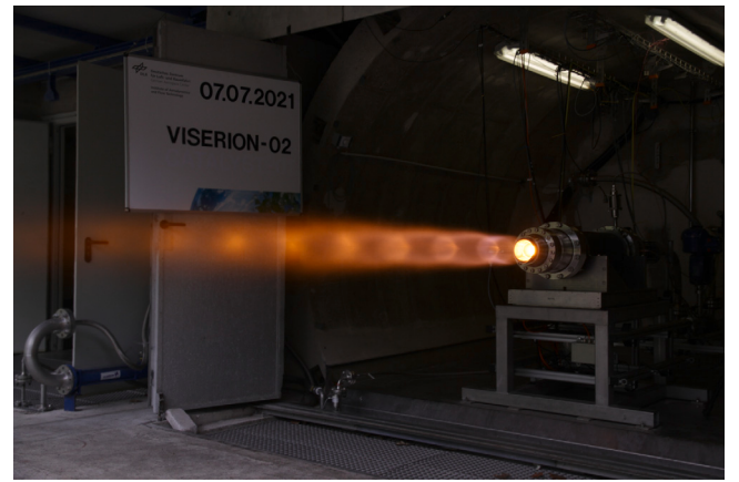
Fig. 10. Full engine test of the VISERION engine [36].
