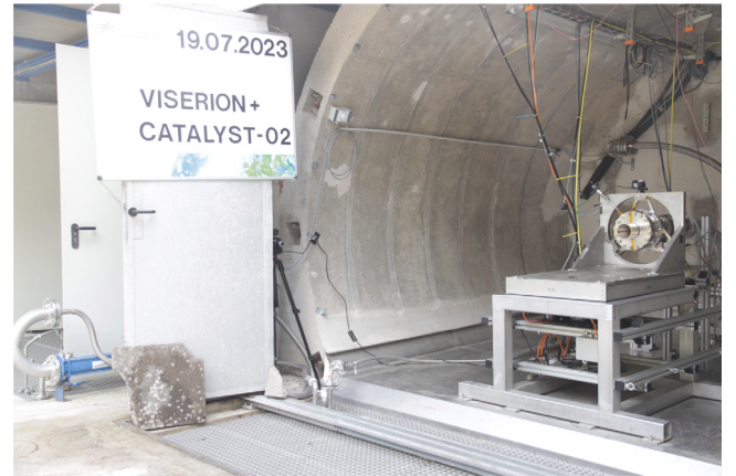
Fig. 9. Catalytic chamber test of the VISERION engine.
