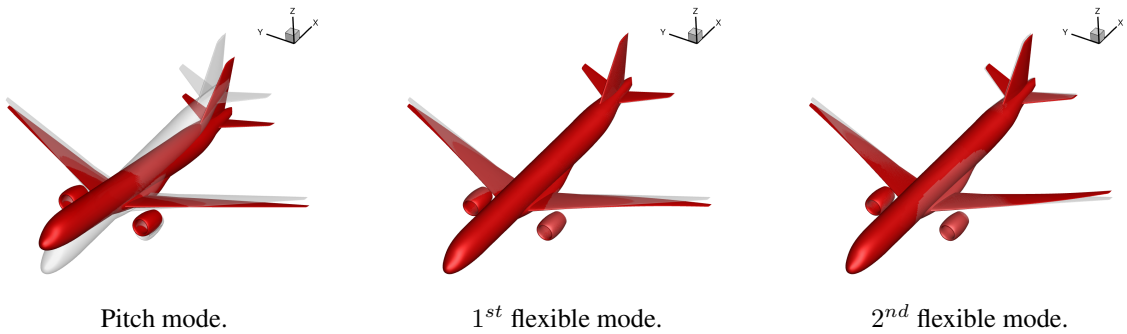
Figure 2: Example of structural eigenvectors splined to the CFD surface.
