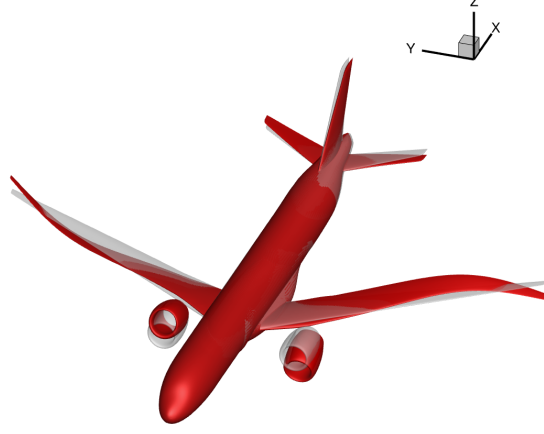
Figure 4: Flutter mechanism of the DLR-F25 at Mach=0.78 for the considered mass case.
