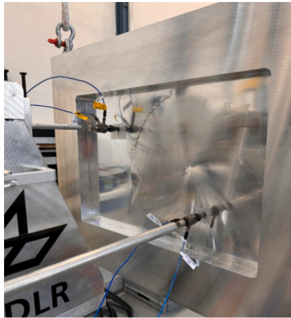
Fig. 5.2. Experimental two-shaker setup (left) and attachment connector (right).
