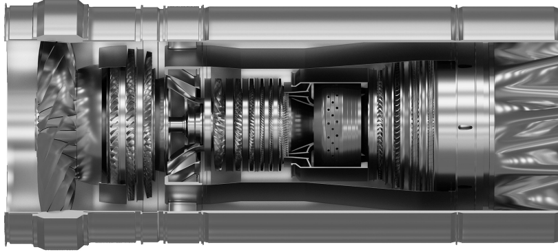
Figure 1.3: Cutaway of the Boom Supersonic Symphony engine design study, source: Boom Supersonic
