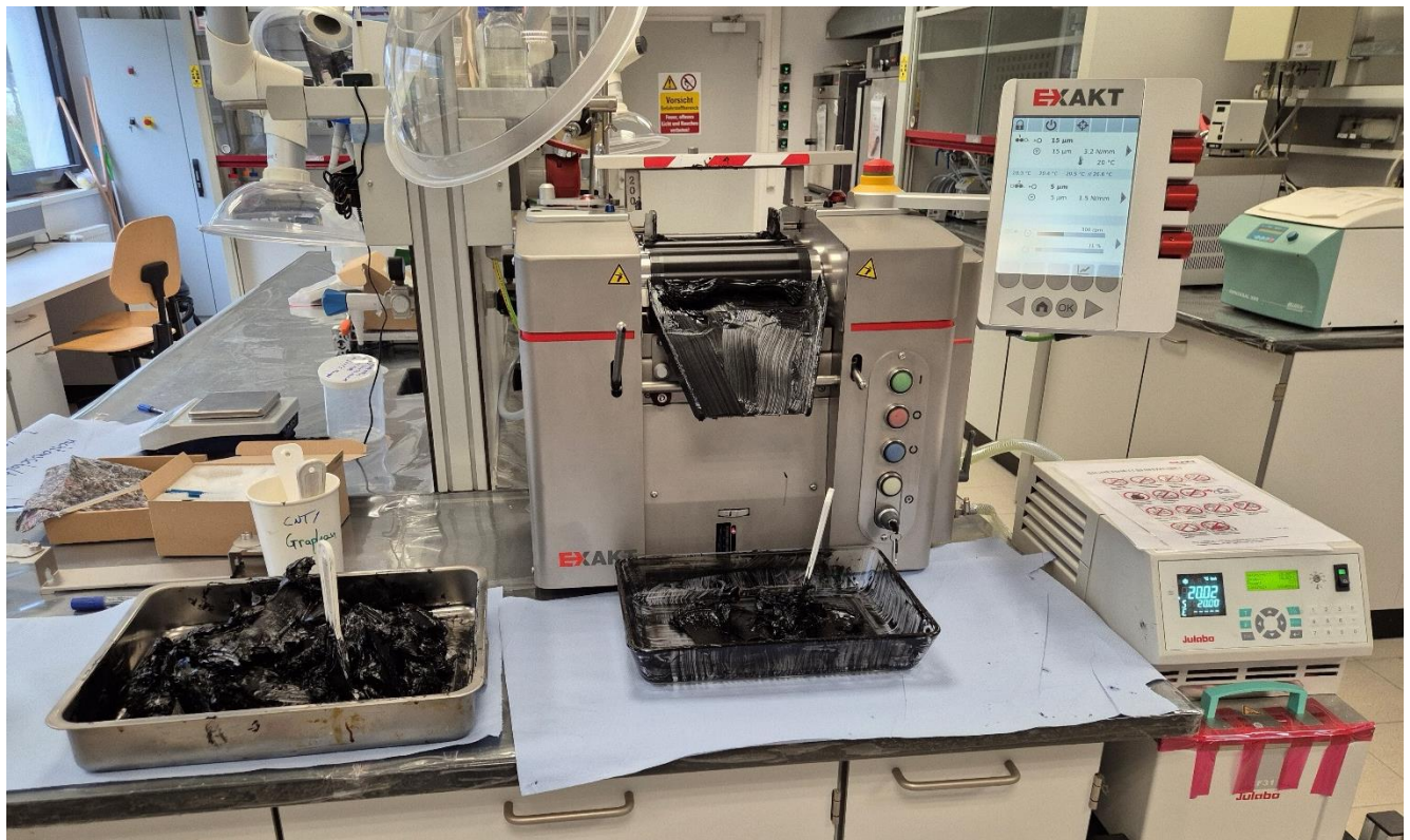
Figure 5-3 – MWCNT dispersion setup using the three-roll mill
