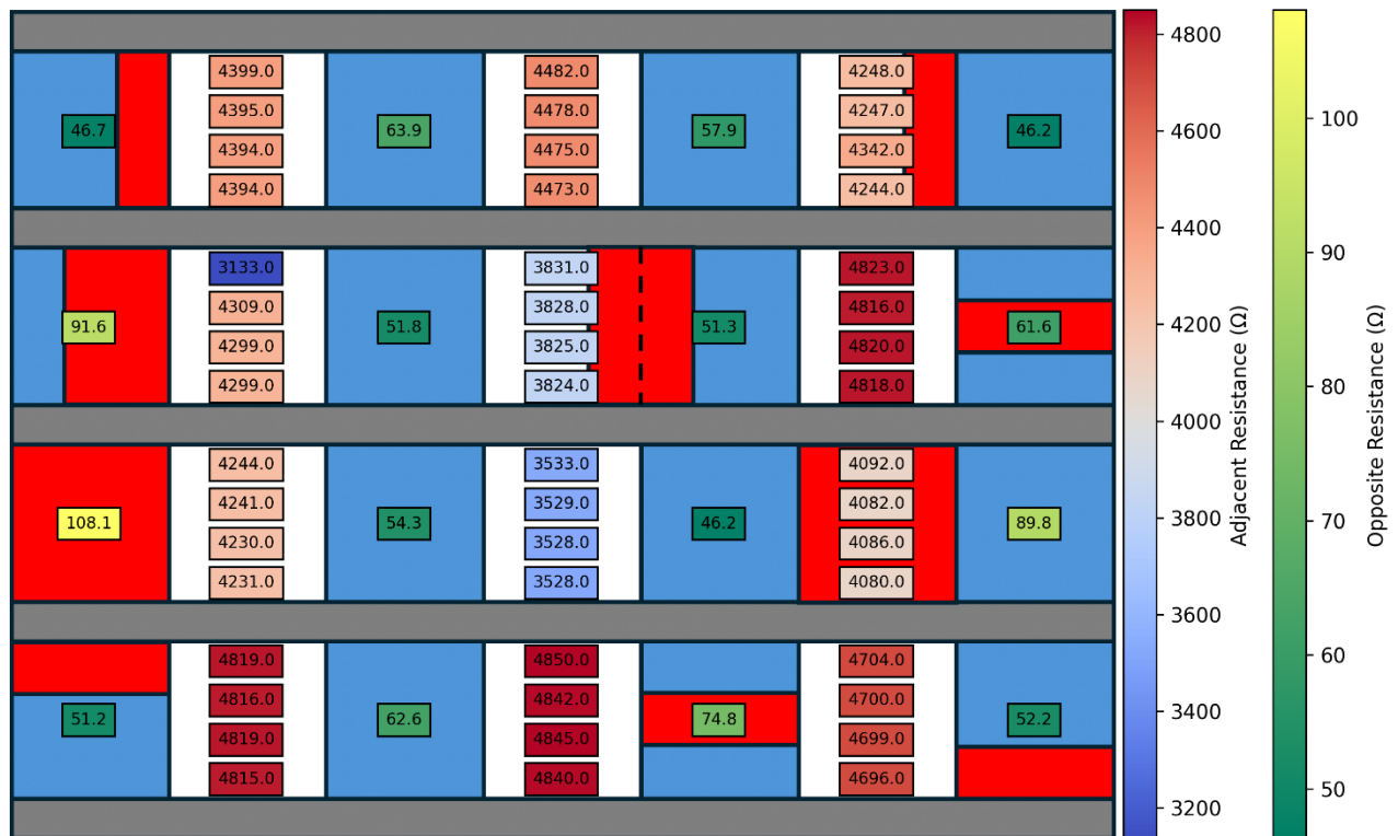
Figure 6-15 – Cohesive failure resistance measurements overlaid onto schematic of the demonstrator
