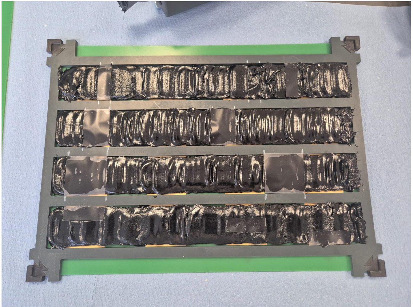
Figure 5-16 – Demonstrator part during glue up with foil and 3D printed part visible
