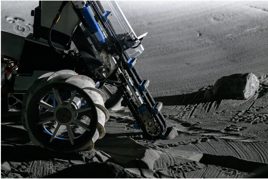
Figure 2.3: Bucket elevator used in the SRC for excavation by Team BREMEN, Photo: ©ESA
