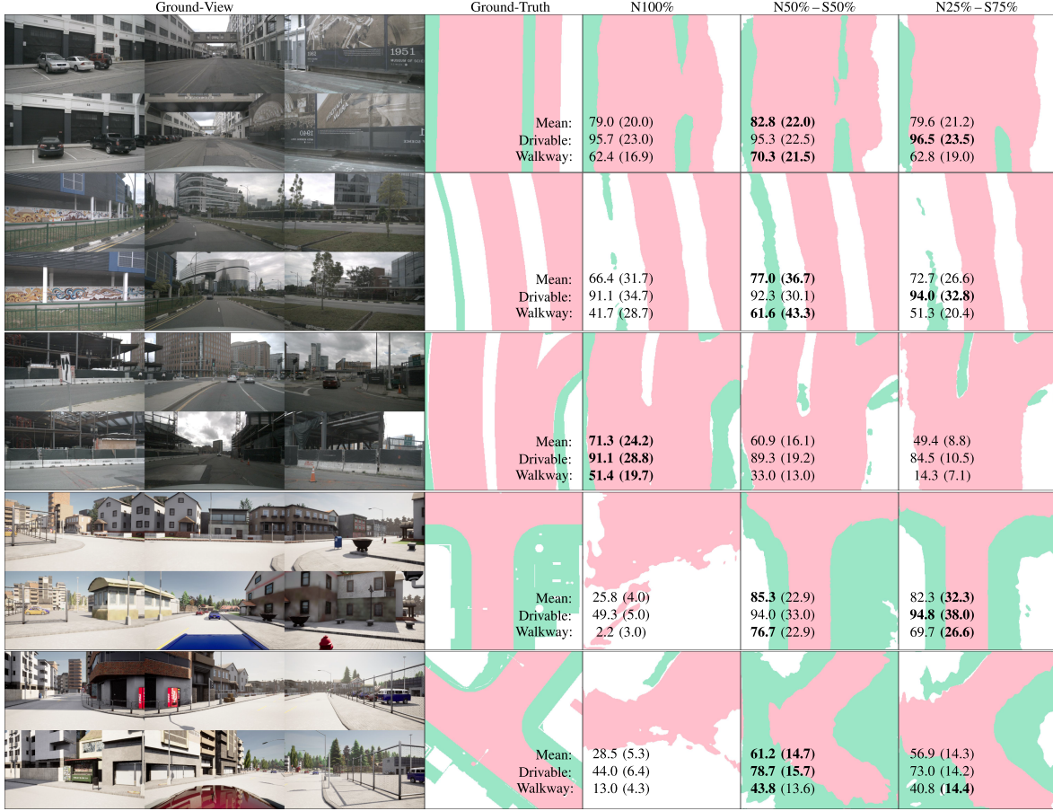
Fig. 10. BEVCar: Qualitative comparison across three samples from the nuScenes dataset and two samples from the synthetic dataset with 30 \times 30 m coverage. On the left is the ground-view, followed by the ground-truth and predictions from models trained on different percentages of real and synthetic data. Drivable area in ■ and Walkway in ■ . We also include quantitative measures for the different predictions including mean and class-wise (boundary) IoU.
