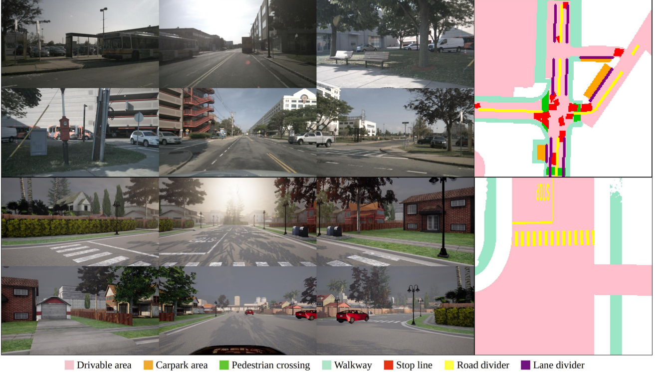
Fig. 1. Samples from the nuScenes (top) and Synthetic (bottom) datasets: ground view (left) and 100 \times 100 \text{ m}^2 BEV map (right). In the ground views, the top images show the front of the ego-vehicle and the bottom images show the rear. The color in the synthetic sample represents all kinds of road markings.
